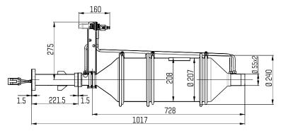
Spread of box dimensions ± 3 mm due to tolerance. Drawings with detail and connection dimensions as PDF and DXF can be found at www.HATZ-DIESEL.com.
